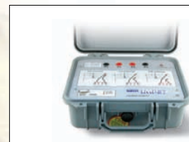
IMP57 Accessory for measuring loop impedance with high resolution
