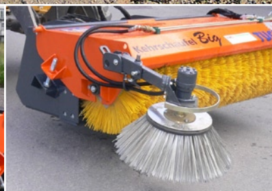
Fully adjustable hydraulic side brush (50% PP / 50% wire)
