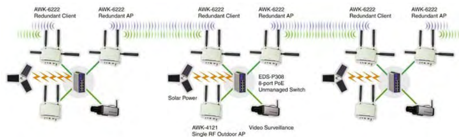
Fig. 1. Suitable WLAN communications equipment includes Ethernet switches and IP cameras with EN50155 and EN50121-1/2 certification to confirm their resilience in harsh railway environments, plus hardened wireless devices.
