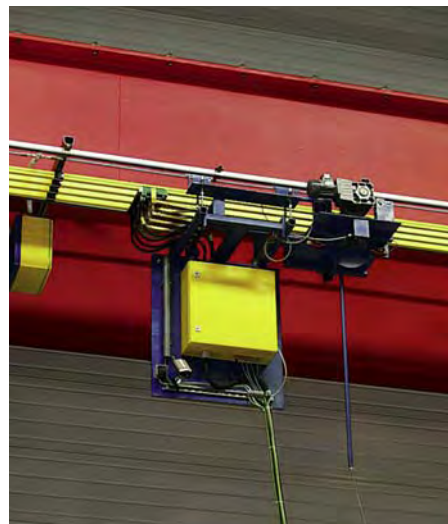
Loop conductors with co-located leaky feeder provide data and power to the production line from above
