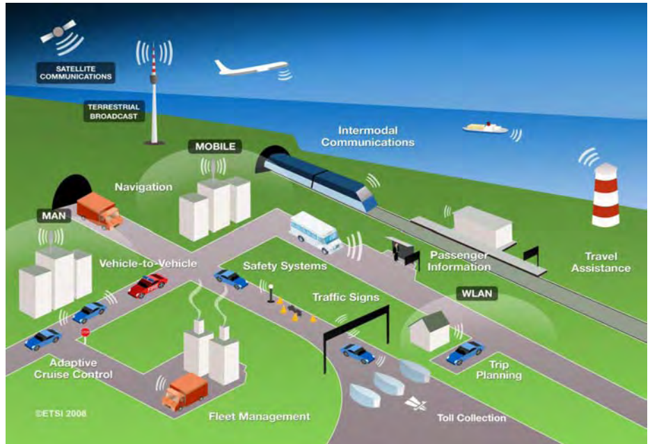
Fig. 1. Intelligent Transport Systems (ITS) include all types of communications in vehicles, between vehicles and between vehicles and fixed locations. Such systems include the use of information and communication technologies (ICT) for rail, water and air transport (picture ETSI).
